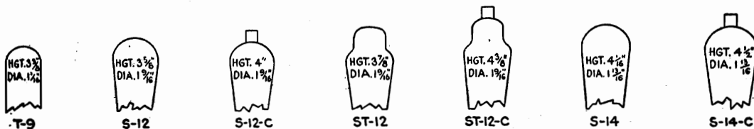
BULB ILLUSTRATIONS—HGT. Designates Maximum Height of Tube when SEATED IN SOCKET.
