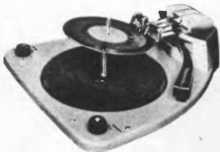
A. To play 7-inch small-hole records, press down on the RECORD SUPPORT RELEASE and move the RECORD SUPPORT to the extreme outward position. Rest the records on the ledge of the RECORD SUPPORT and on the off-set of the small spindle.
