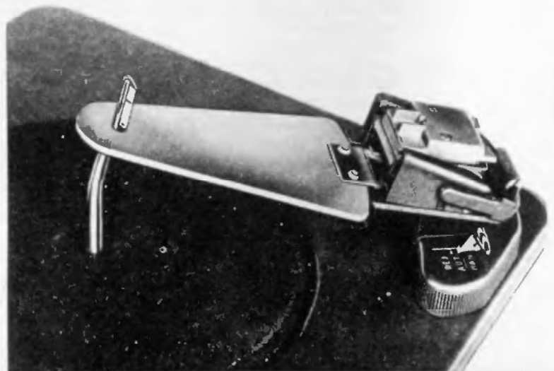
FIGURE 7. SPECIAL RECORD-SHELF GAUGE, SHOWN IN CORRECT POSITION
