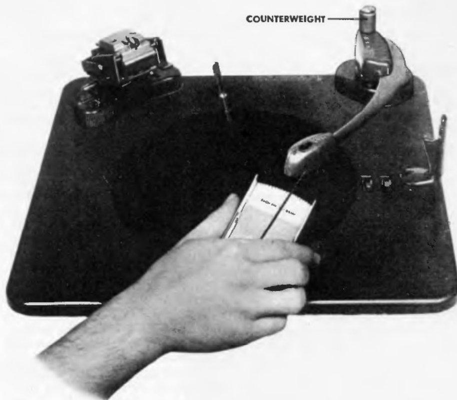
FIGURE 10. MEASURING HORIZONTAL FRICTION
