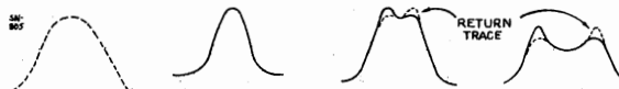
Curve "A" Input to I-F grid. Curve "B" Input to 1st-det. grid, fidelity switch at position 4 (from left). Curve "C" Input to 1st-det. grid, fidelity switch at position 5 (from left). Curve "D" Input to 1st-det. grid, fidelity switch at position 6 (full clockwise).
