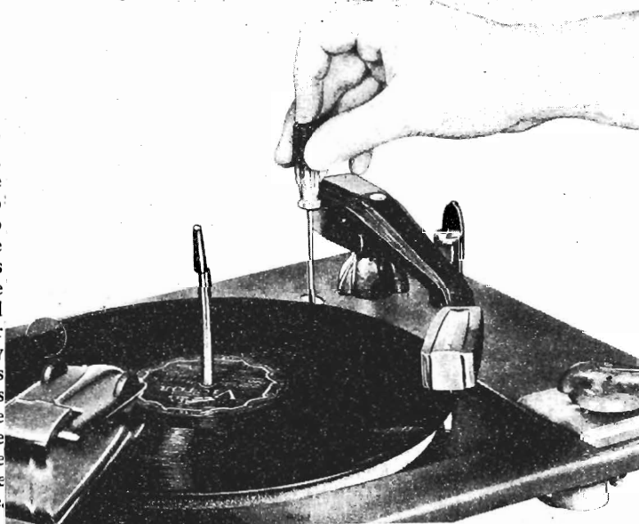
Figure 7—ADJUSTING TONE-ARM SET-DOWN.
