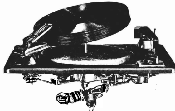
Figure 3—CHANGER, LOADED WITH TWELVE 10" RECORDS.
