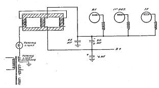
Fig. 13.—Simplified schematic of the tuning indicator circuit of the Majestic 300 series.
