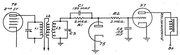
Fig. 8.—Shadowmeter circuit of the Philco model 201.
