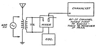
The RF-IF probe is used when aligning the r-f system and also when adjusting the oscillator padder.
