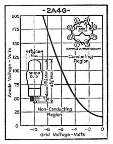
Fig. 3.—Grid voltage-plate voltage characteristic of the 2A4G Thyratron rectifier.
