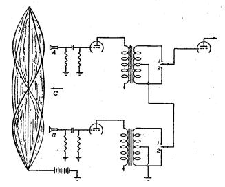
Fig. 2.—Positions of pick-ups in relation to the vibrating string and their output circuits.
