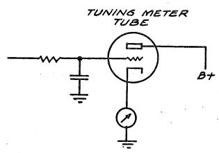
Fig. 4.—Here the tuning meter is at ground potential and the I.R. drop across the meter resistance supplies bias for the tube.
