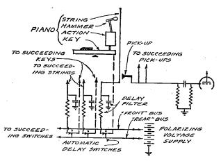
Fig. 1.—Relation of piano action, pick-ups and automatic delay switches.
