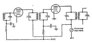
Fig. 5.—By using this arrangement, a separate tuning meter tube is not required.
